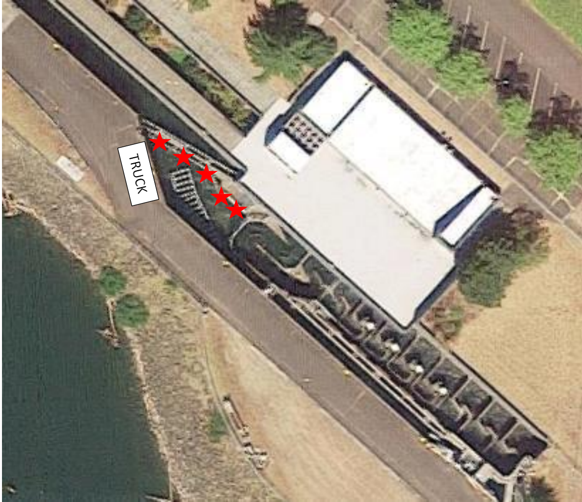
Figure 4. Close-up aerial view of the Bonneville Dam Washington Shore Fish Ladder at the count station and visitors center. Potential trap locations above picket leads are denoted by red stars. Alternate locations may be selected upon consultation between USACE and CRITFC member Tribes.
