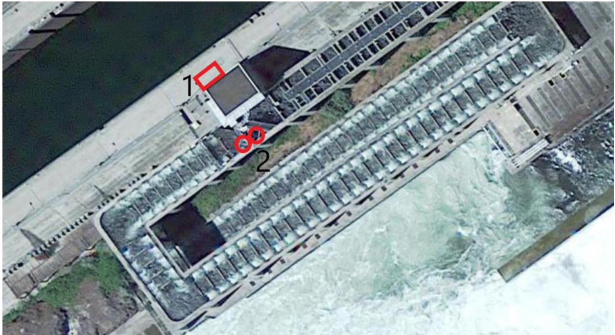
Figure 11. Close-up aerial view of the JDA North Fish Ladder. Red circles (2) denote the location of tube traps deployed above picket leads in the fishway.
