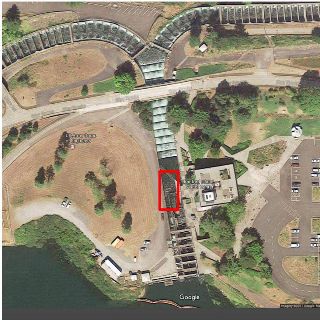
Figure 5. Close-up aerial view of the Bonneville Dam Bradford Island Fish Ladder at the count station and visitors center. Potential trap locations above picket leads are outlined by red box. Alternate locations may be selected upon consultation between USACE and CRITFC member Tribes.
